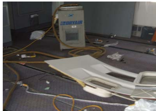
Heat Exchangers on the main deck, with and without air ducting attached
