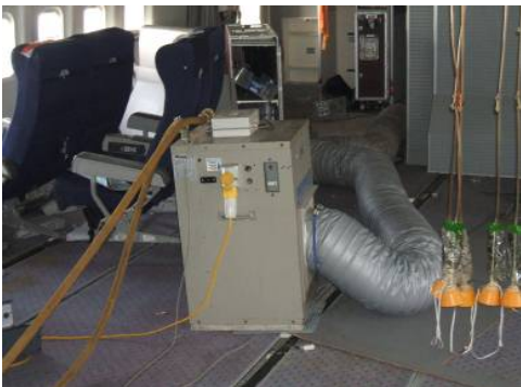
Heat Exchangers on the main deck, with and without air ducting attached
